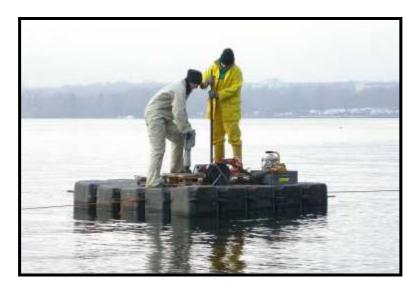
Figure 55: Taking cores from the drilling platform at Lake Wannsee.
