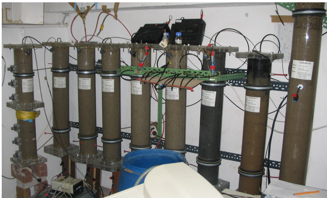
Figure 102 Short retention columns at the DWQC at the TU Berlin
