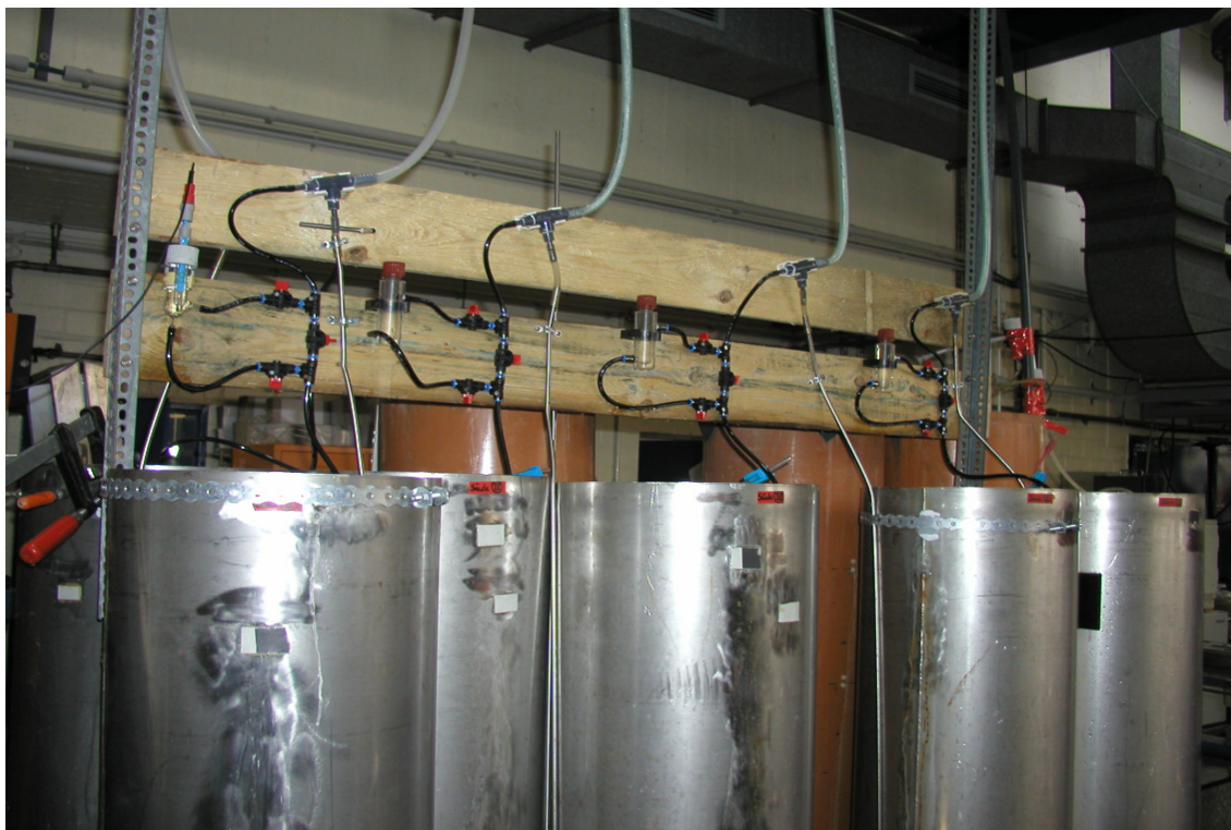
Figure 70 Long retention soil columns Marienfelde (top part)
