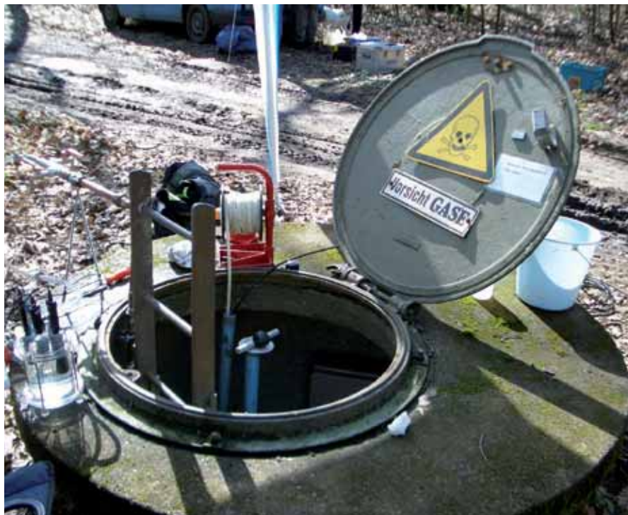
Diagnosis campaign at selected wells: Hydrochemical and microbiological analyses
