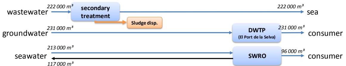
Figure 2-3: Overview of the LCA scenarios for El Port de la Selva and annual water volumes
