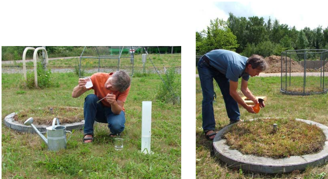
Fig. 29: Spiking of glyphosate on lysimeter: dosing of the herbicide (left) and spraying of the herbicide onto the lysimeter surface (right)
