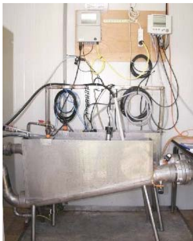
Figure 2.5: Measurement flume for sewer and discharge channel (left) and sampling equipment set-up (right) (Graner et al. 2007)
