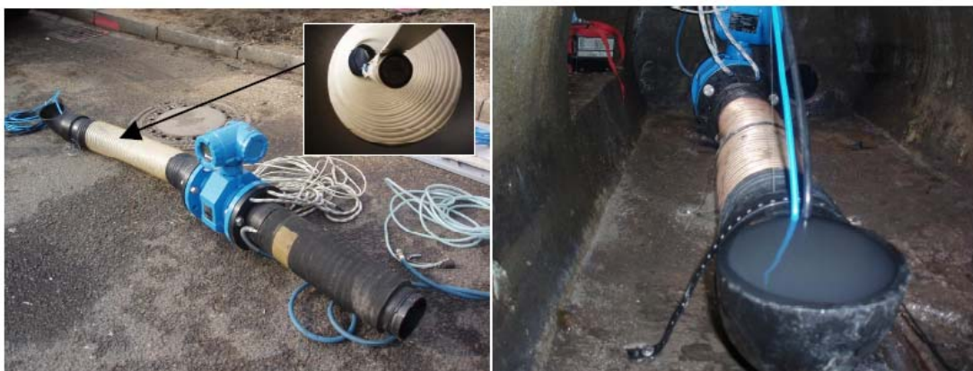
Figure 2.11: Water quality parameter and flow measurement in the sewer system (temporarily measuring point) (Hoppe et al. 2008)
