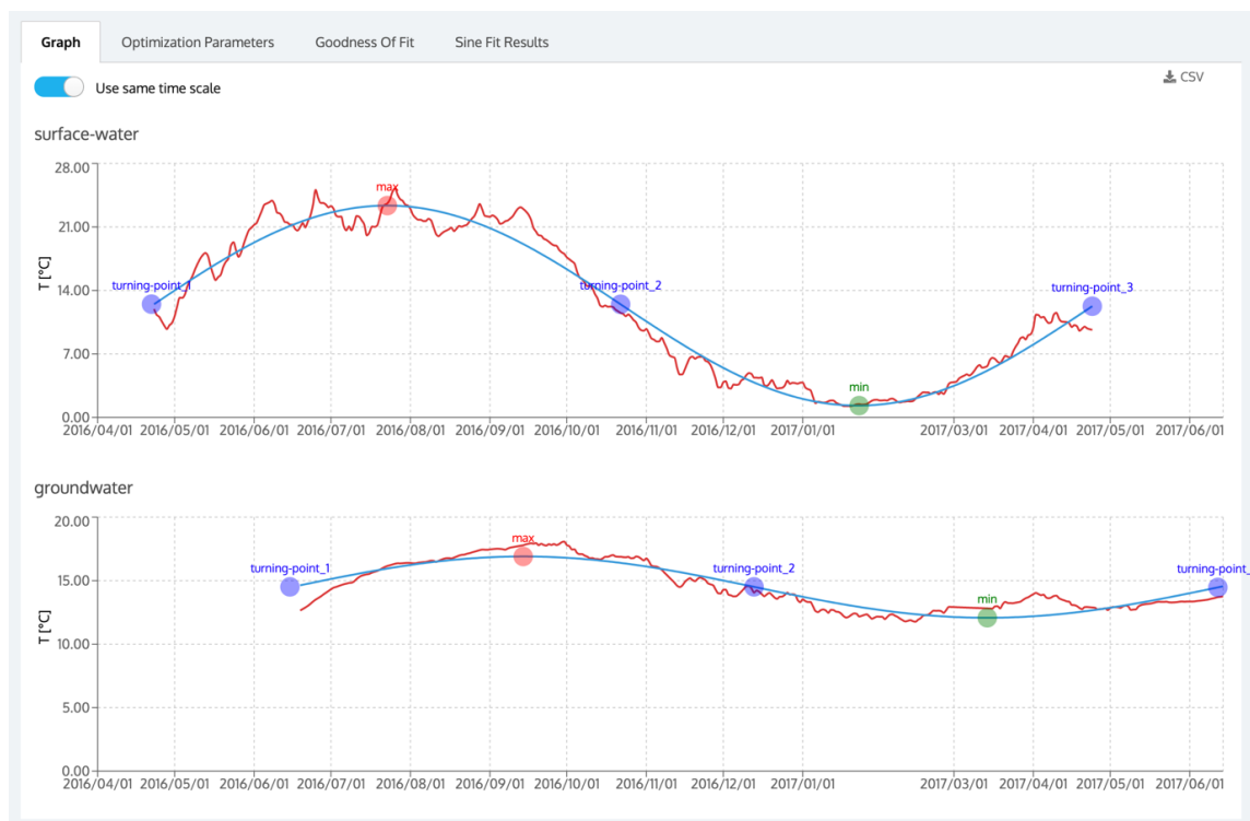
Figure 5. Calculation results: graphic visualisation of sine curve fitting with display of calculated min/max and turning points for surface water and groundwater time series
