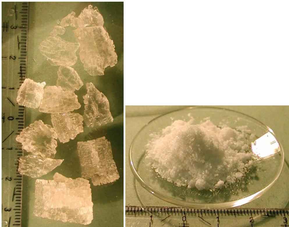
**Picture 11:** Stercorit ( $\text{H}(\text{NH}_4)\text{Na}(\text{PO}_4) \cdot 4\text{H}_2\text{O}$ ) washed crystals and grinded washed crystals from self crystallization from concentrated urine
