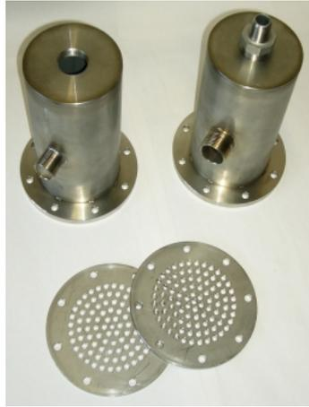
Connecting sockets and perforated plate
