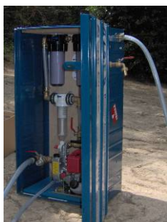
Figure 17 - Own treatment system designed by GSCF
