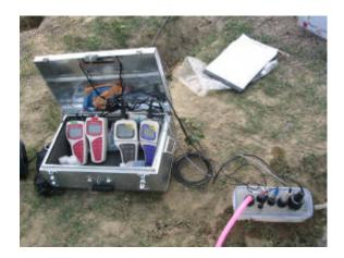
Figure 4.14 Measuring in-situ paramters on site (flow-through cell, measuring devices in steel box).
