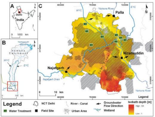
**Figure 4.4** A: Overview India. B - Spatial extent of the Yamuna catchment upstream of Delhi and course of the Western- (WYC) and Eastern Yamuna Canal (EYC). C - Location map of the three selected field sites with trends in groundwater flow directions and isobath depths of groundwater.
