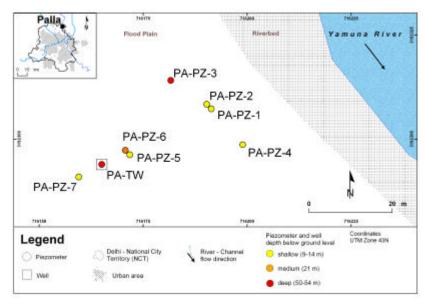
Figure 4.8 Piezometer setup in Palla.
