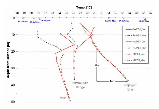
Figure 4.18 Temperature logs from the months of December 2006 and May 2007, showing actual temperature gradient in the deepest piezometers of each field site. Surface water temperatures of adjacent water bodies and temperature gradient at Najafgarh Drain are also indicated.
