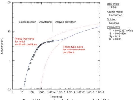
Figure 4.16 Neuman solution for the drawdown period at PA-PZ-6.
