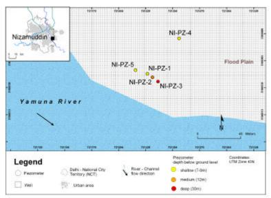
Figure 4.12 Piezometer setup at Nizamuddin bridge.
