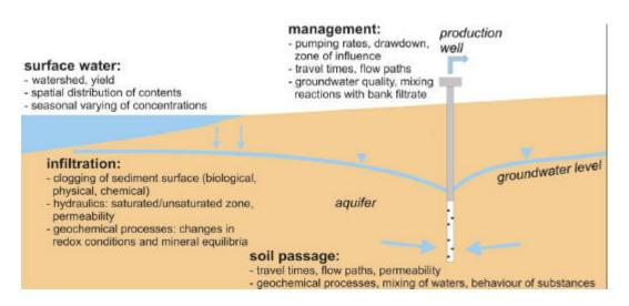
Figure 3.1 Sketch of factors influencing bank filtration (modified from FRITZ 2002)
