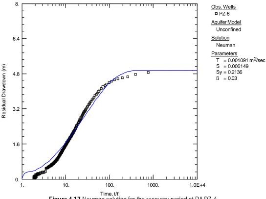
Figure 4.17 Neuman solution for the recovery period at PAPZ-6.
