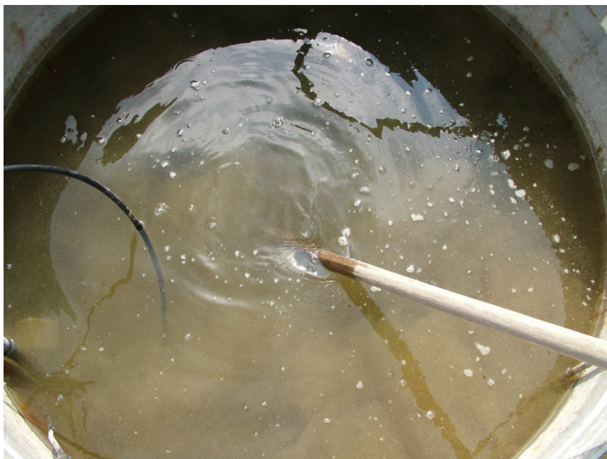
Figure 58: Gas bubble formation during removal of clogging layer on enclosure III in December 2004.
