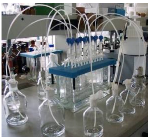
Figure 1. Picture shows the build up of a solid phase extraction
