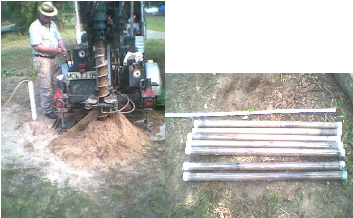
Figure 1: Snap shot of NORDMEYER drill (left) and recovered plastic liner containing aquifer sediment (right).
