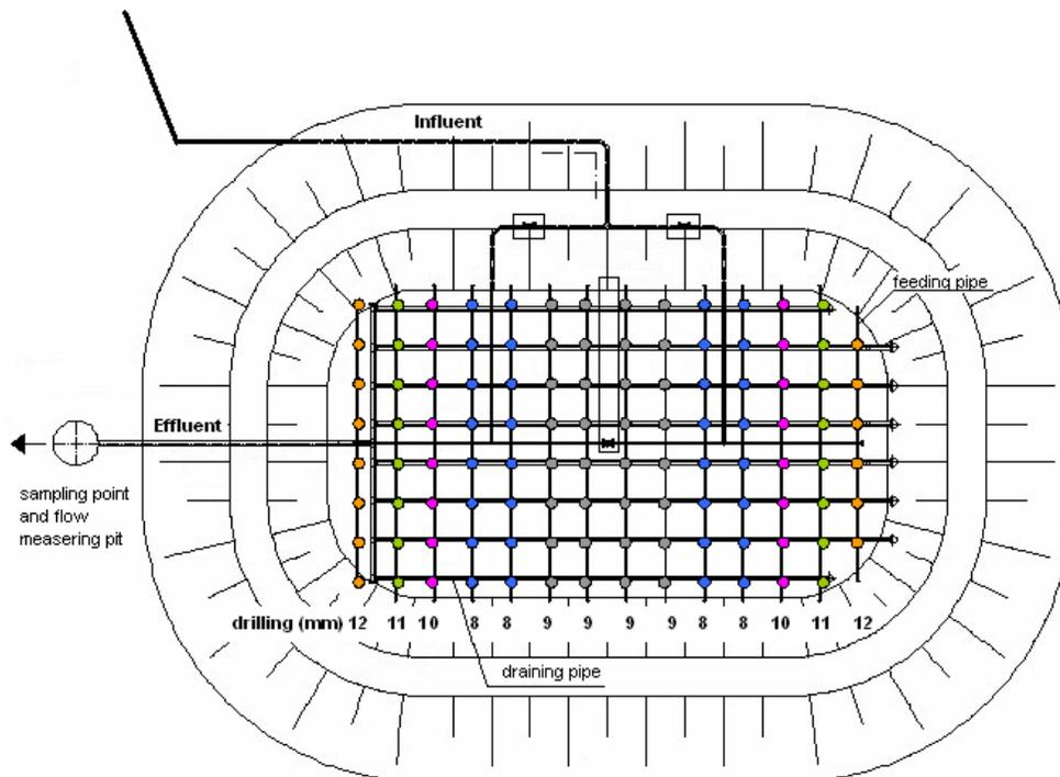
**Fig. 2.4.17:** Constructed wetland, distribution system
