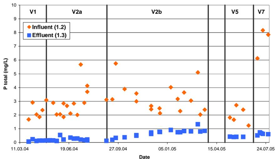
**Fig. 3.5.6.6:** Total phosphorus concentration of the influent and effluent of the constructed wetland (24 h composite sample)
