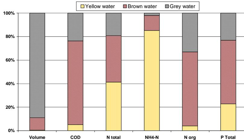
**Fig. 3.6.1:** Volume and mass balances of different parameters of yellow, brown and grey water (data basis: yellow water: *Variant V1 to V7*; brown water: *Variant V2b*; grey water: *Variant V5*)
