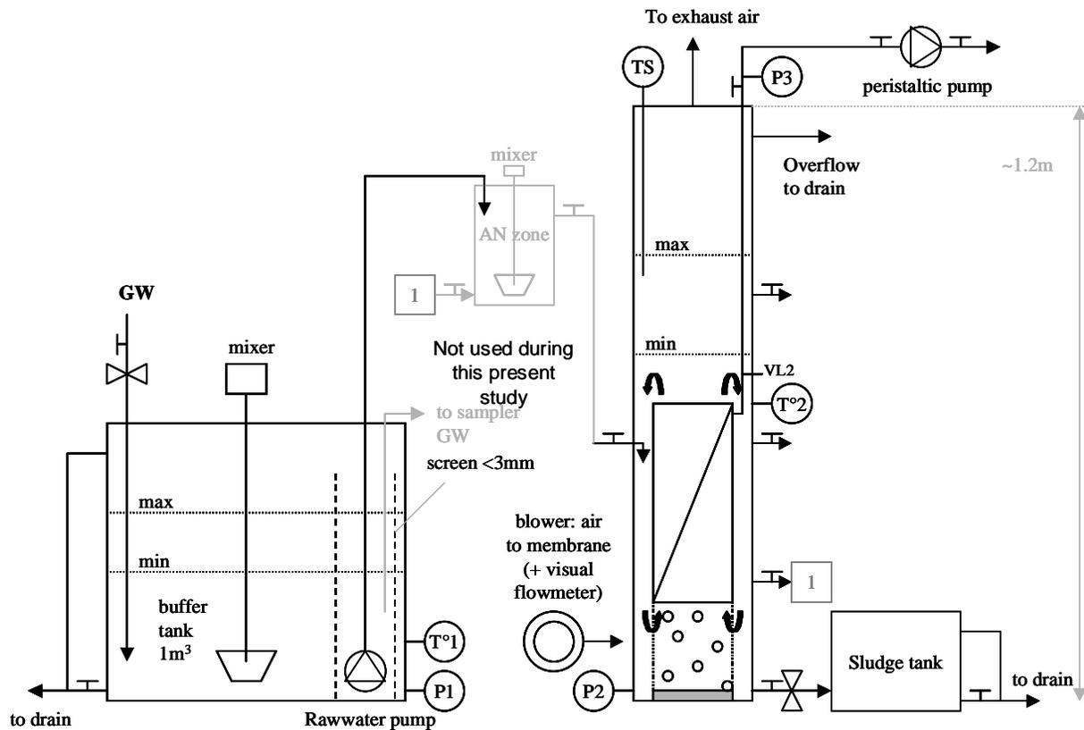
**Fig. 2.4.8:** Flow scheme of the membrane bio-reactor
