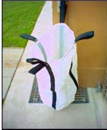
**Fig. 2.4.9:** Fugafil-Saran Filter bag (PE 1200/500) for faeces dewatering
