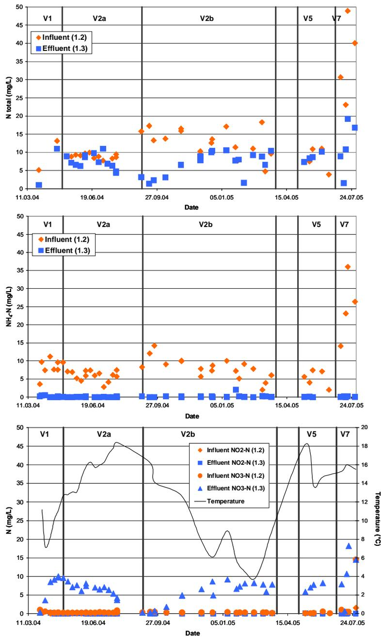
**Fig. 3.5.6.5:** Nitrogen parameters of the influent and effluent of the constructed wetland (24 h composite sample) (above: N-total; middle: NH<sub>4</sub>-N; below: NO<sub>2</sub> and NO<sub>3</sub>)
