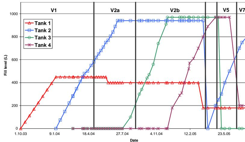
**Fig. 3.4.1:** Fill characteristic of the urine tanks and storage time of the urine from the office building
