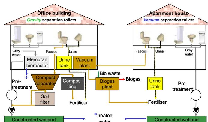
**Fig. 6.1:** New sanitation concepts with *gravity* separation toilets in the office building and with *vacuum* separation toilets in the apartment house of the WWTP Stahnsdorf
