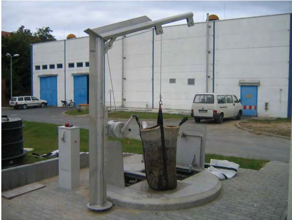
**Fig. 2.4.11:** Faeces dewatering facility including crane
