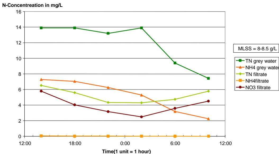
**Fig. 3.5.7.2:** Evolution of nitrogen concentration in grey water and filtrate during 24 hours
