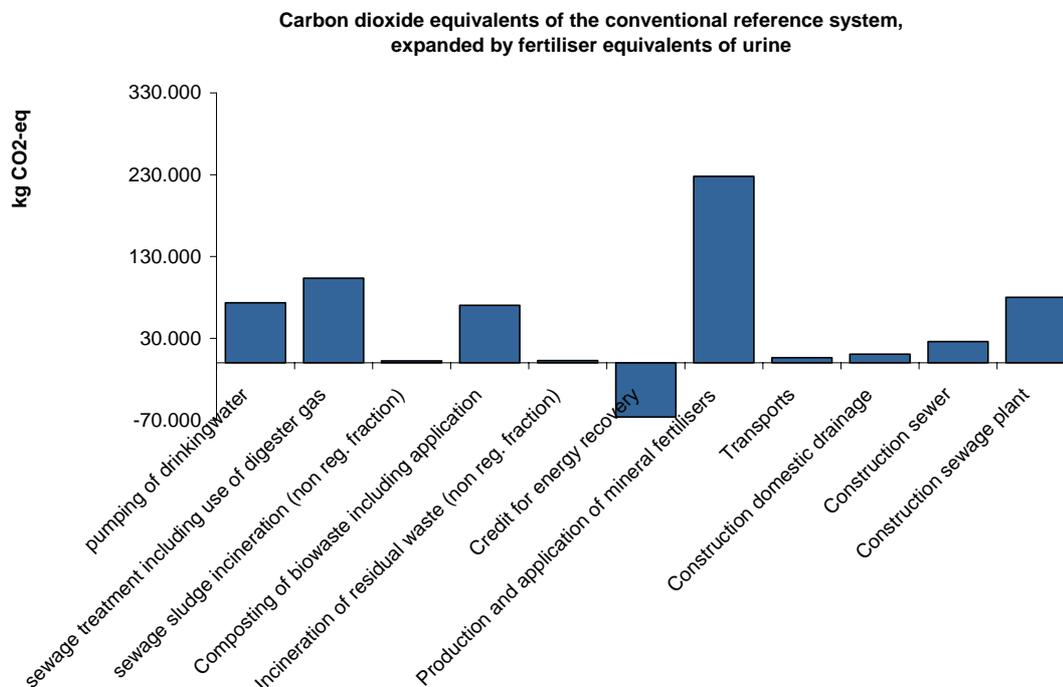
Fig. 10: carbon dioxide equivalents of the conventional reference system, expanded by fertiliser equivalents of urine
