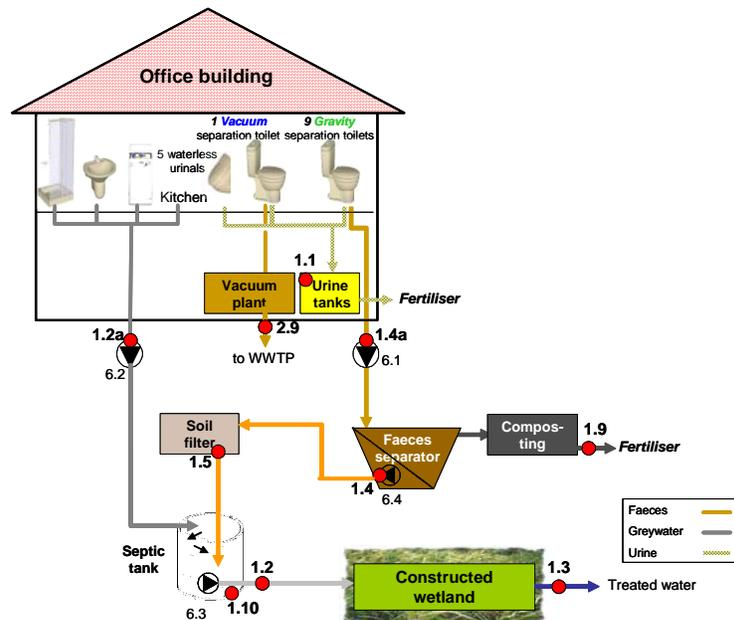
**Fig. 2.3.3:** Flow scheme of *Variant V1* (with soil filter)
