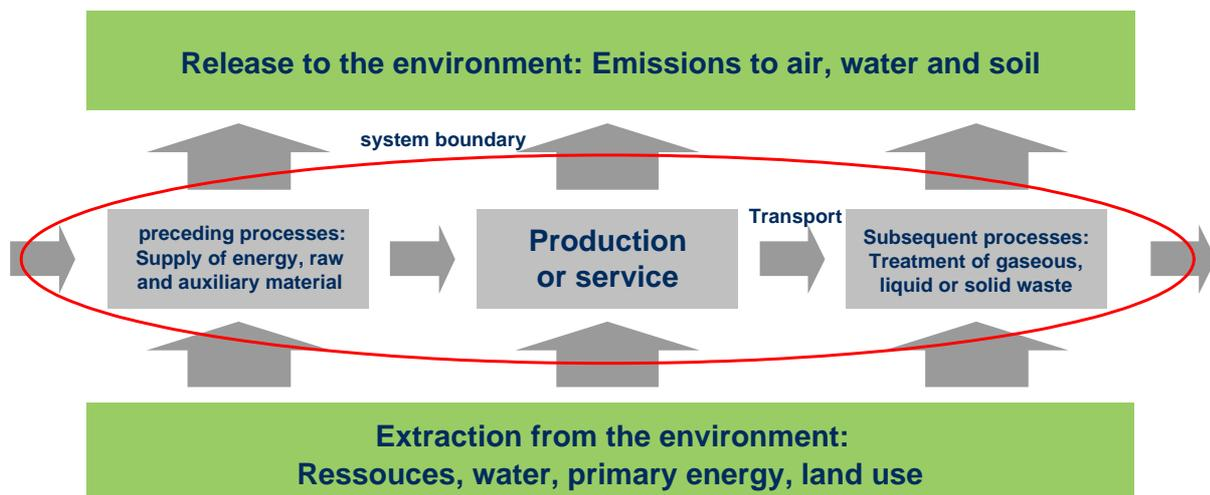
Figure 2: Simplified structure of a LCA-system
