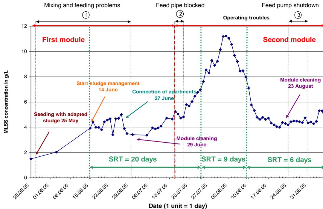
**Fig. 3.5.7.1:** MLSS evolution in the reactor and operational conditions
