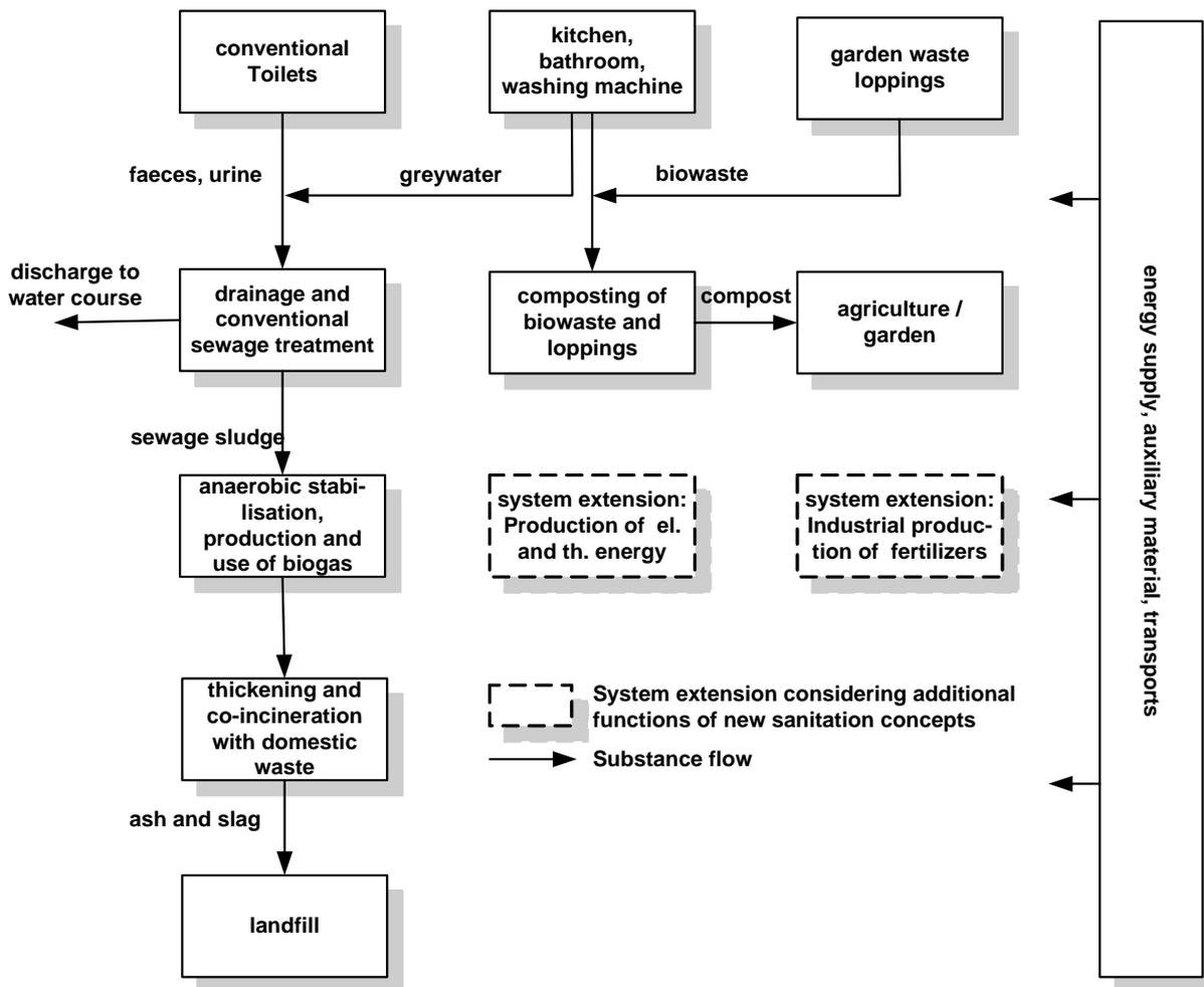
Fig. 4: Conventional system for reference of comparison (variant 1)
