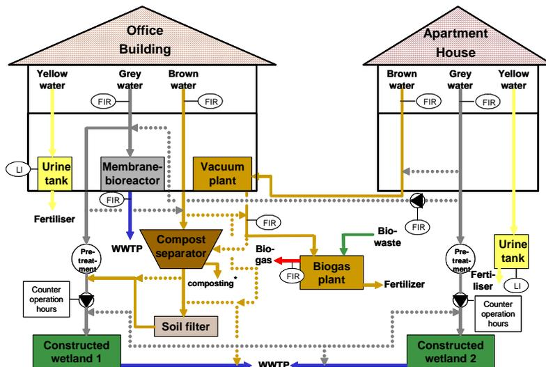
**Fig. 2.1.2:** New sanitation concepts with *gravity* separation toilets in the office building and with *vacuum* separation toilets in the apartment house of the WWTP Stahnsdorf
