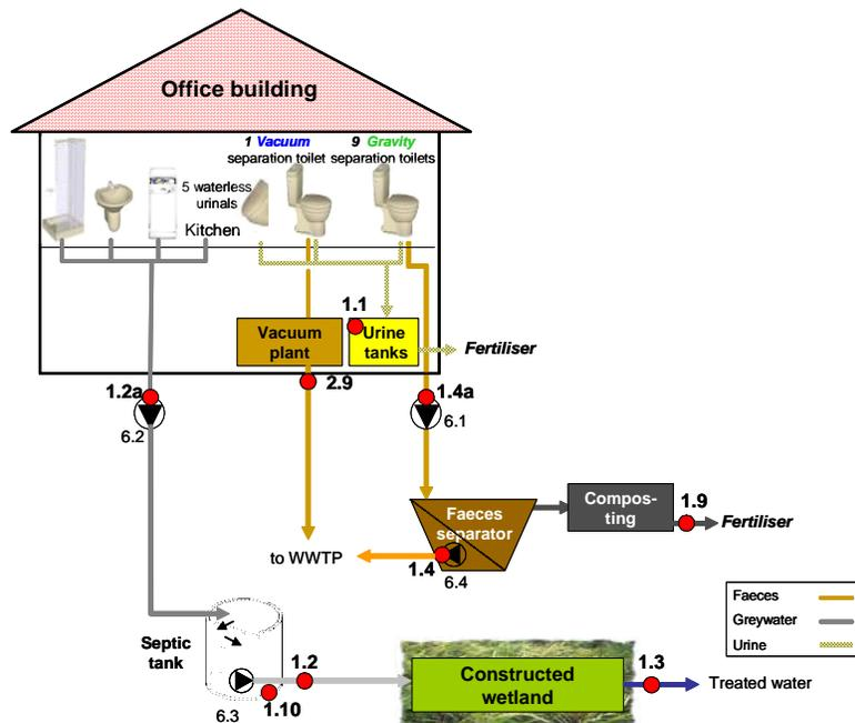
**Fig. 2.3.4:** Flow scheme of *Variant V2a* (without soil filter and no treatment of faecal filtrate)
