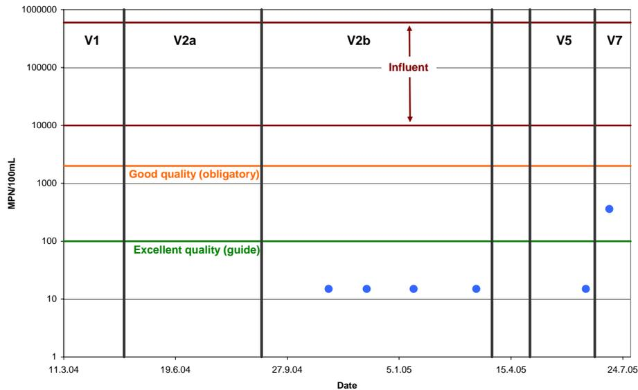
**Fig. 3.5.6.8:** Faecal coliforms in the influent and effluent of the constructed wetland
