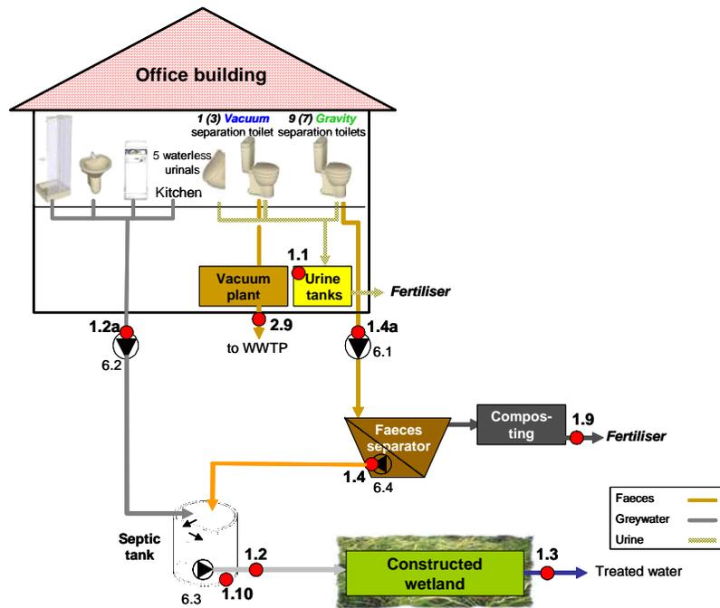
**Fig. 2.3.5:** Flow scheme of *Variant V2b* (without soil filter, but treatment of faecal filtrate)
