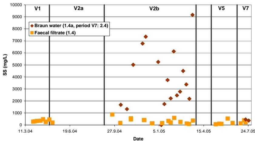
**Fig. 3.5.2.2:** SS concentrations of brownwater in the infl. and effl. of the faeces separator during the different variants (24 h-composite samples)(1.4, 1.4a and 2.4 are samplings points, see **Fig. 2.3.7**)
