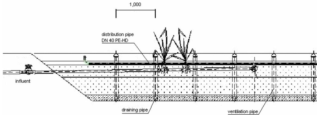
**Fig. 2.4.16:** Constructed wetland, cross section
