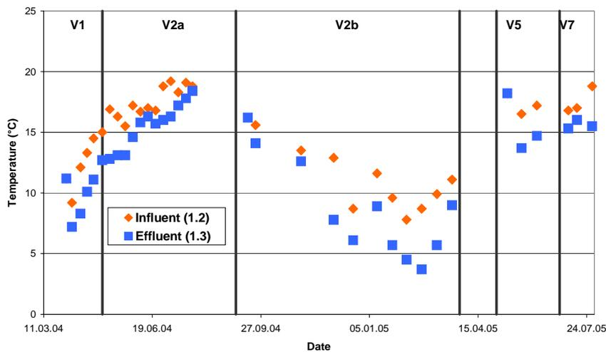
**Fig. 3.5.6.2:** Temperature of the influent and effluent of the constructed wetland
