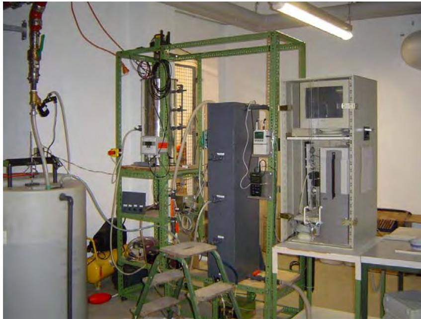
**Fig. 2.4.6:** Membrane bio-reactor
