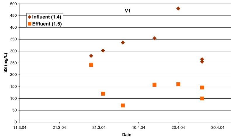
**Fig. 3.5.4.1:** Influent and effluent SS-concentration of the soil filter (24 h composite sample)
