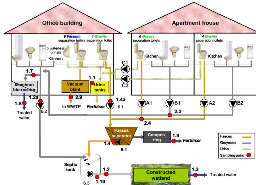
**Fig. 6.3:** New sanitation concepts with *vacuum* separation toilets in the office building and with *gravity* separation toilets in the apartment house of the WWTP Stahnsdorf
