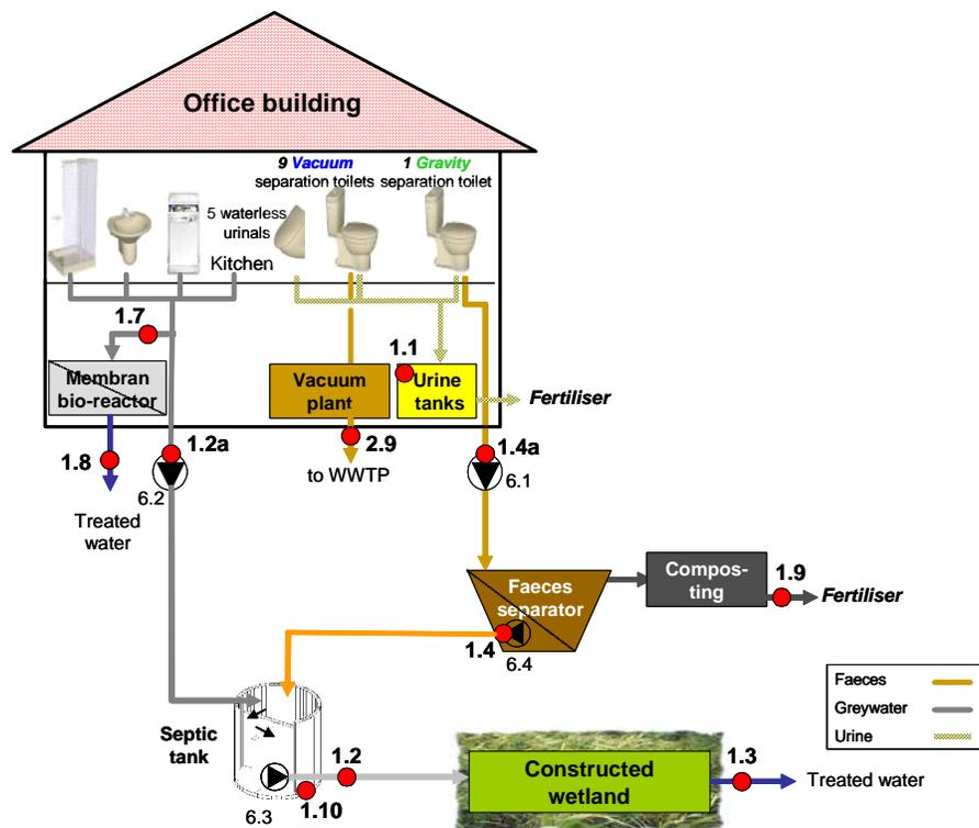
**Fig. 2.3.6:** Flow scheme of *Variant V5* (without soil filter, but treatment of faecal filtrate and operation of membrane bio-reactor)
