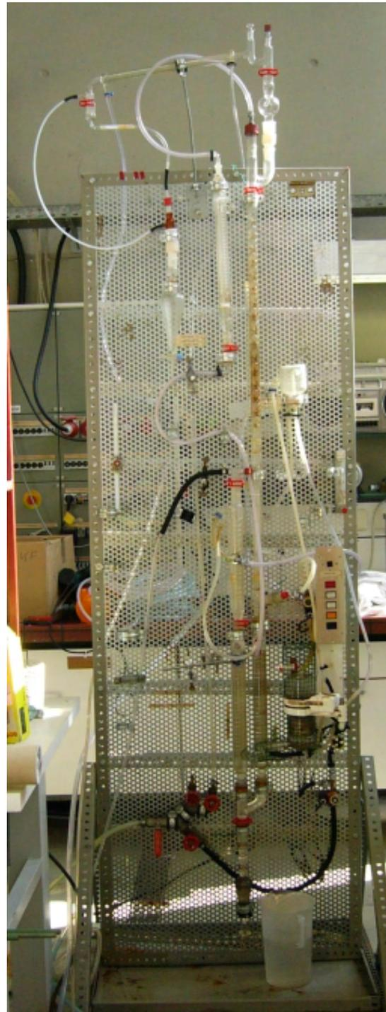
**Picture 6:** Steam stripping unit in laboratory scale
