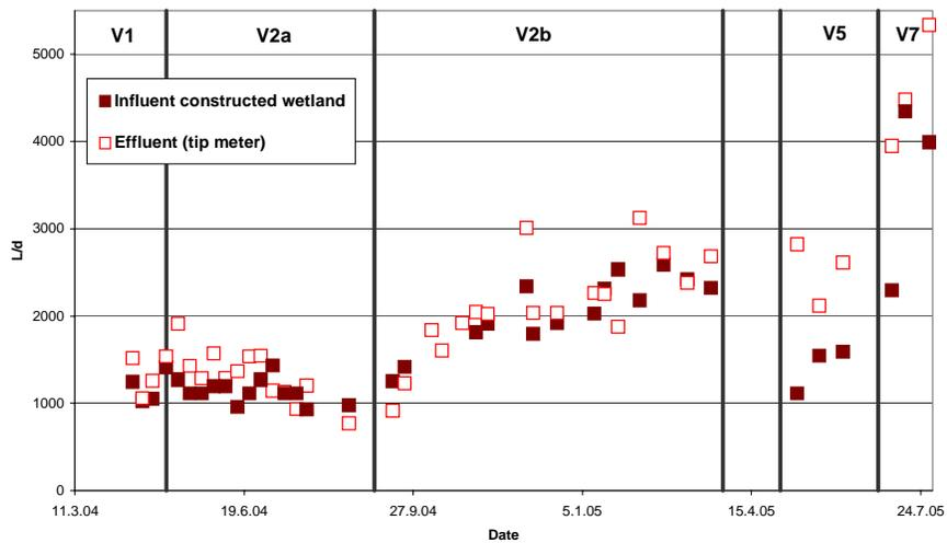
**Fig. 3.5.6.1:** Influent and effluent flow of the constructed wetland
