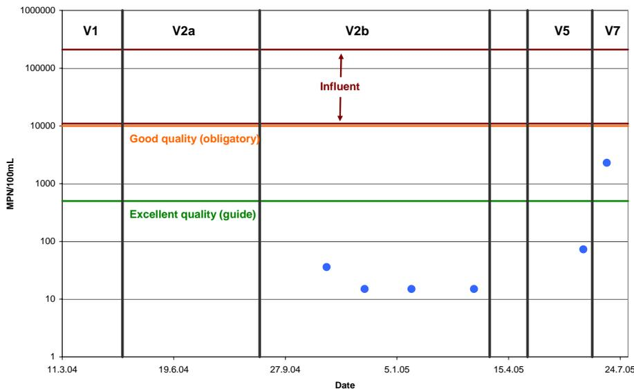
**Fig. 3.5.6.7:** Total coliforms in the influent and effluent of the constructed wetland
