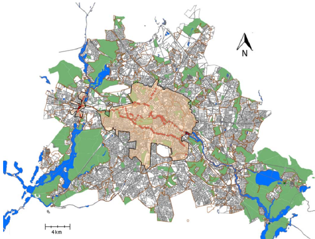
Figure 2: Map of the city of Berlin, the combined sewer system and its waterways. The River Spree crosses the city centre flowing from south-east to north-west. The light red area represents the part of the city drained via a combined sewer system. Red dots indicate the position of CSO outlets along the Spree and its side-channels.
