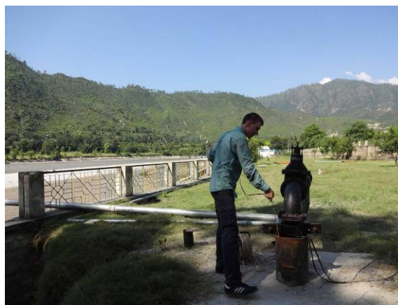
Fig. 4-4 Pumping test and sampling being conducted on MW4 & PW4 (Photo: V.D.A. Nguyen, HTWD, September 2012)
