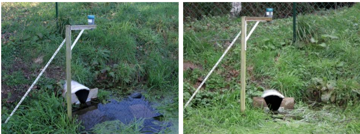
Figure 18: Measurement of outflow in surface wetland.
