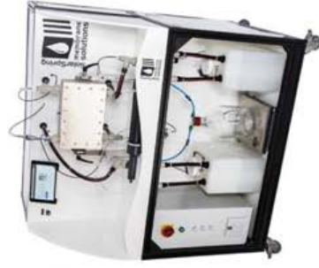
MD bench scale experimental set-up
