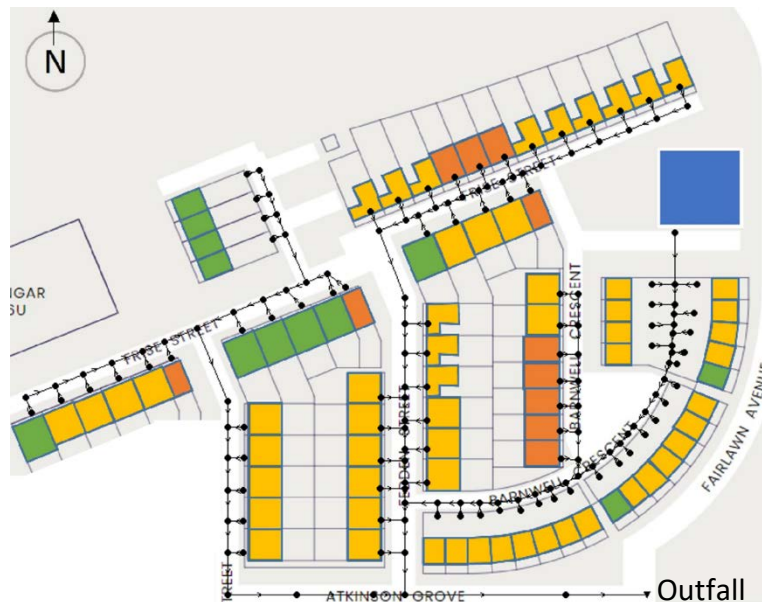
Figure 13 Map of the development with overlaid sewer network adapted from YTL Developments (113 housing units).
