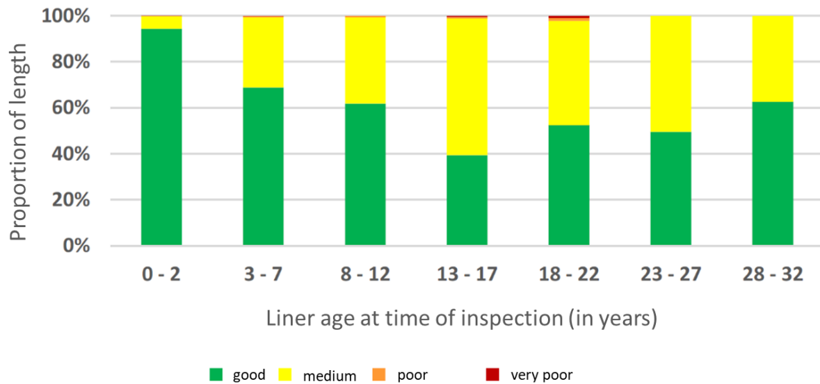
Figure 8: Condition distributions (ordinate) of the evaluated liners for the liner age groups at the time of inspection (abscissa); Figure from BWB
